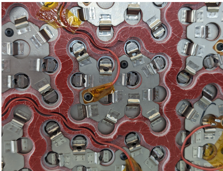
Figure 31: Ring Terminal PCB on segment
