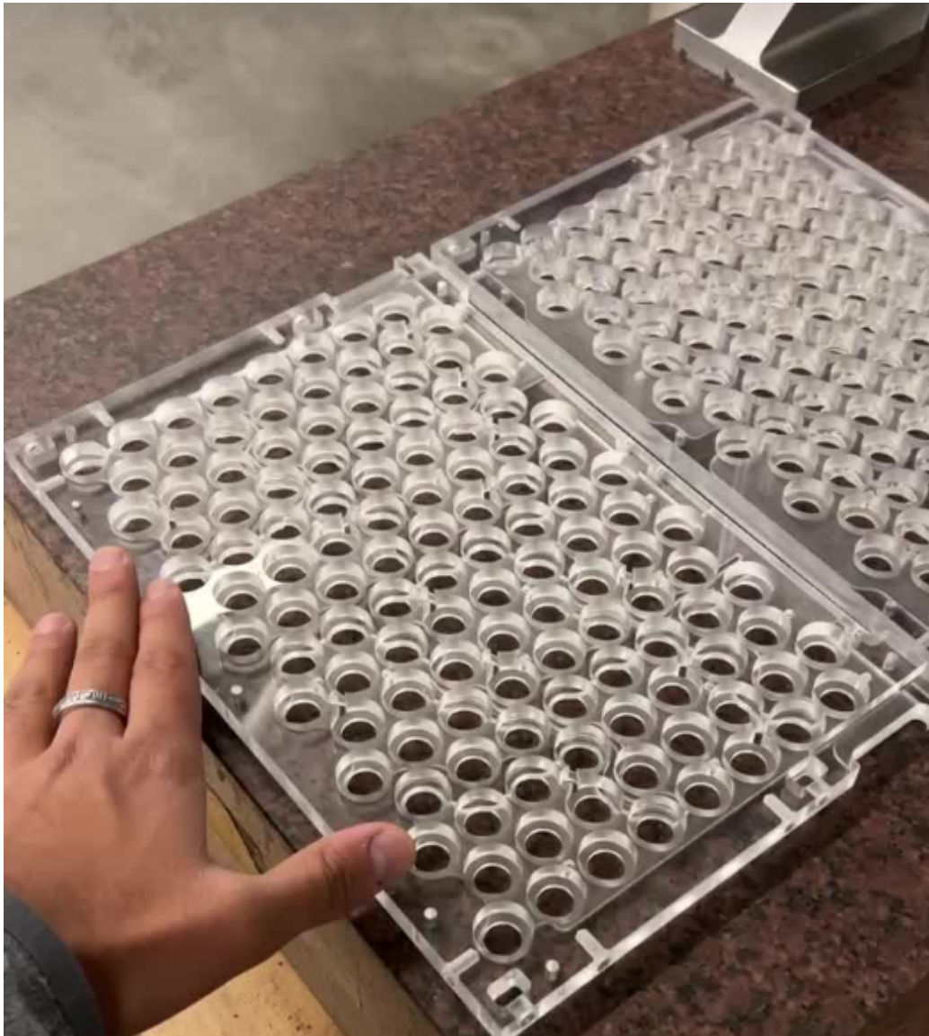
Figure 30: Lexan Segment Walls
