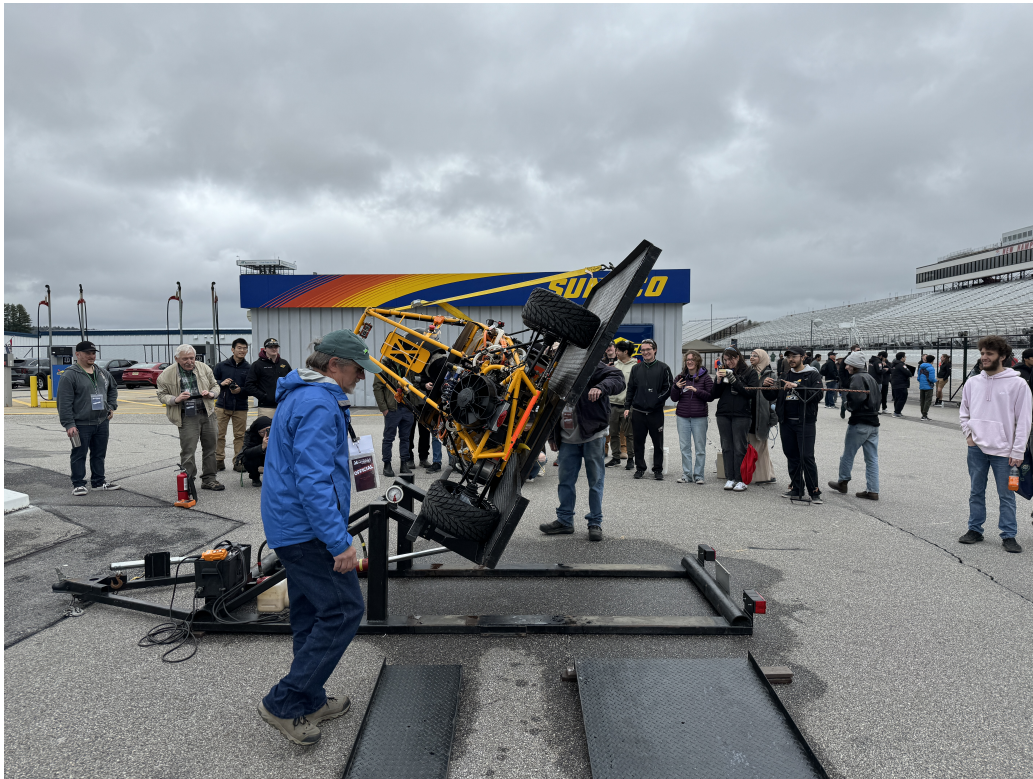
Figure 13: Demonstration of failed tilt test of vehicle (note visibility under right rear wheel)
