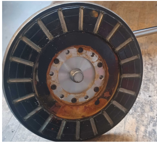
Figure 3: Permanent Magnet side of Emrax 208 Motor that failed (notice significant orange residue (rust), indicative of water ingress)
