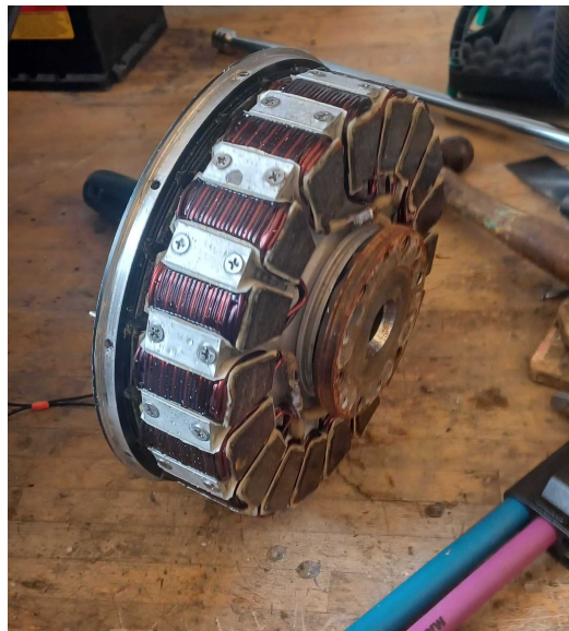
Figure 4: Coil side of Emrax 208, insulation tests showed arcing between case and coils due to insulation degradation around the windings.
